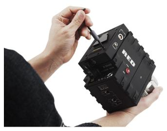
Loosen the screws in an "X" pattern
