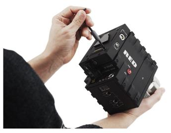
Tighten the screws in an "X" pattern
