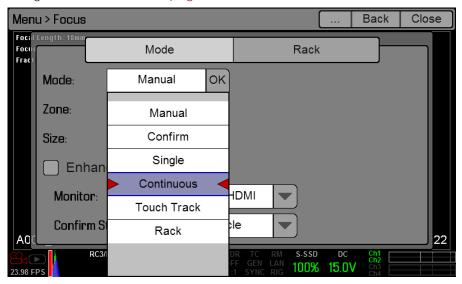
In Single, Continuous, and Touch Track modes, a single target displays on the screen that indicates where the image will be in focus. In Rack mode, multiple targets display on the screen to indicate the different areas between which the camera will rack focus.
