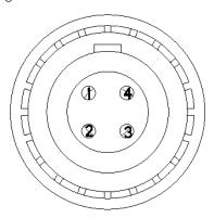
CTRL (RS232) Connector Mating Connector: FGG.00.304.CLAD27Z
