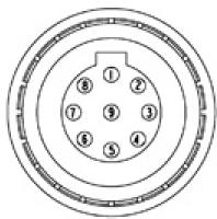
Ethernet Connector Mating Connector: FGG.0B.309.CLAD32Z
