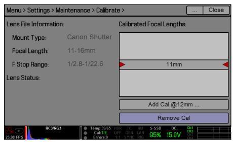
The lens calibration process for the current focal length starts and a progress bar displays. Once the calibration process starts, DO NOT touch the lens, as doing so may cause the lens to calibrate incorrectly.
