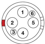
DC In Power Input Connector Mating Connector: LEMO FGJ.1B.306.CWLD72Z
