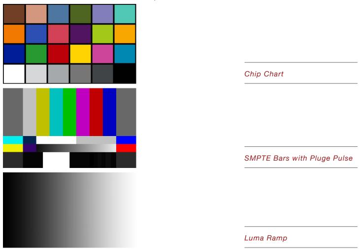
NOTE: RED DSMC test signals are not recordable; they are provided to help align external video monitors connected via the HD-SDI or HDMI outputs.
