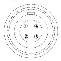
SYNC (Video Sync) Connector Mating Connector: FGG.00.304.CLAD27Z
