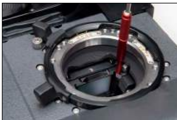
Figure 101: Ground glass in camera with Ground Glass Puller attached
