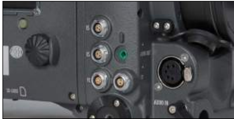
Figure 16: 24 V outputs (RS) and 12 V output
