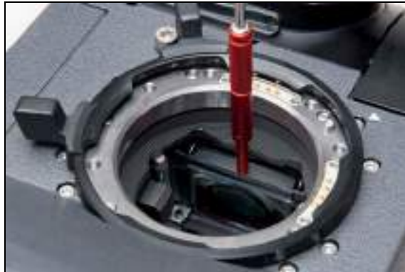
Figure 103: Field lens in camera with attached Ground Glass Puller
